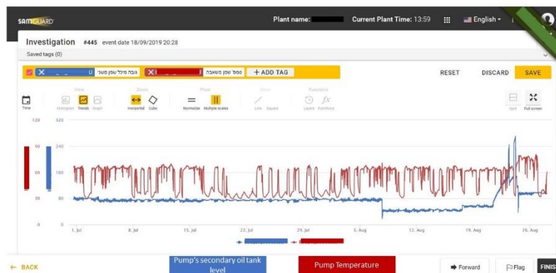
Fig. 3. SAM GUARD sent two alerts that it identified as related to each other: higher-than-usual temperature and higher-than-usual oil level. The two alerts together enabled the engineer to immediately understand the problem and the required action
